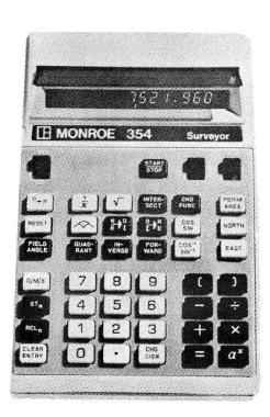
You're looking at the Monroe Micro Surveyor— the very first hand-held battery powered programmable micro computer specifically designed for the surveying professional.
